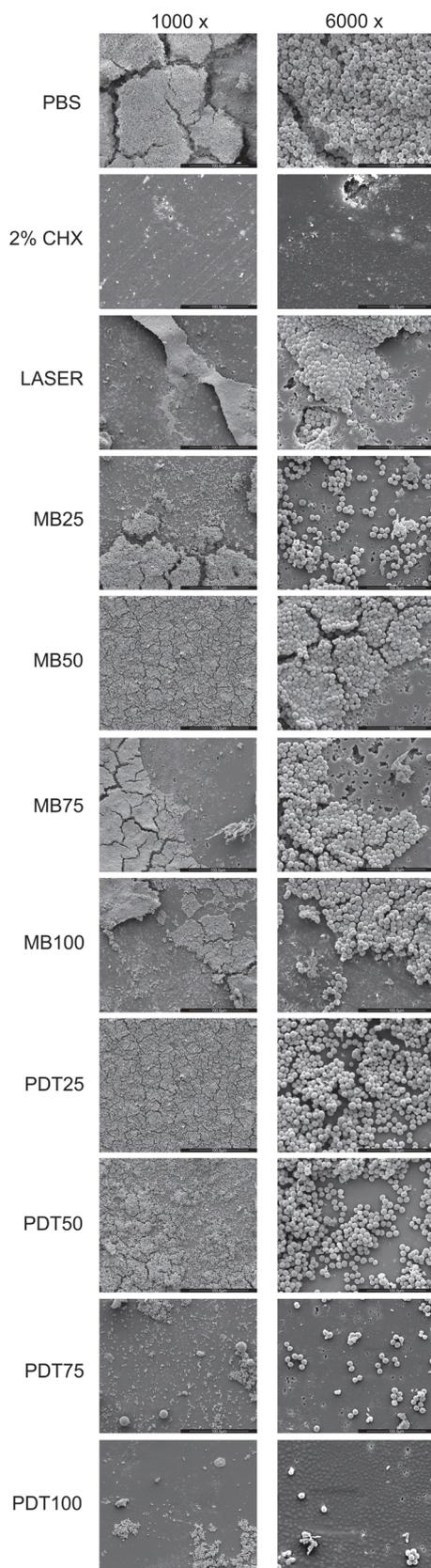
**Fig. 3.** Scanning electron microscopy images at 1000 $\times$  (scale bar =50  $\mu$ m), 6000 $\times$  (scale bar =10  $\mu$ m) of specimens of acrylic resin specific for ocular prostheses colonized by *Staphylococcus aureus* biofilm, immersed in different disinfectant treatments. H<sub>2</sub>O was used as the negative control. WD = 10 mm; 15 kV.
