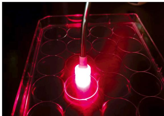
Fig. 1. Irradiation of specimens containing the biofilm using a continuous wave diode laser device.
